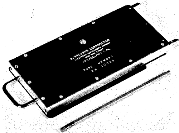
Figure 5b. Rope Memory Package Capacity: 256 Words, 64 Bits per Word.
