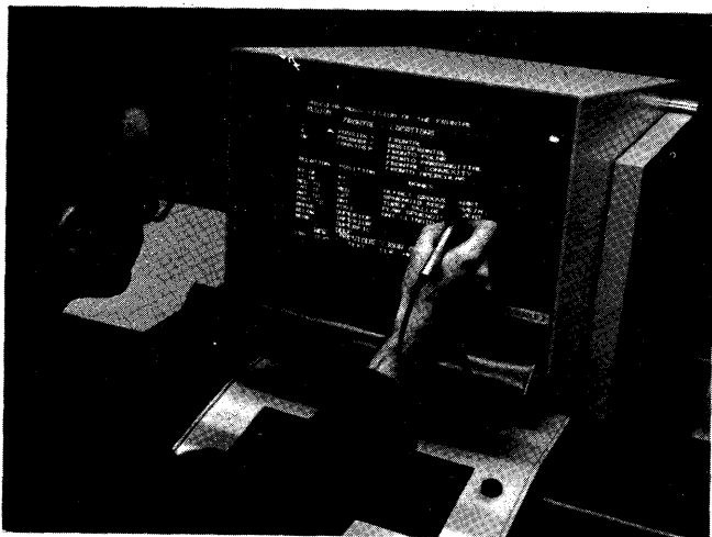
Figure 1.—Display and use of light-pen, with experimental video matrix terminal.
