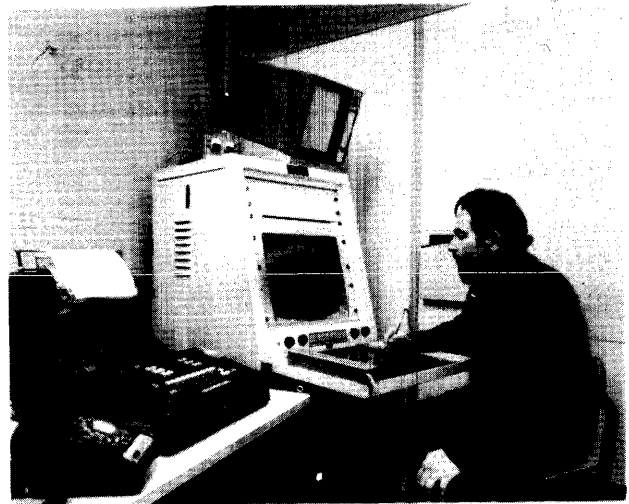
Figure 1—An interactive computer-mediated animation console. The author is sketching with the stylus on the tablet. There is a CRT for viewing dynamic displays, a storage scope above it, a typewriter, knobs, toggle switches, and a telephone so that an animator may summon help
