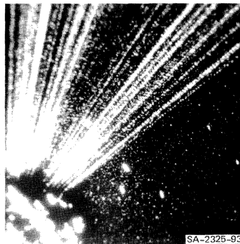
Figure 6—Effect of one-second burst of signal on radar plan-position indicator
