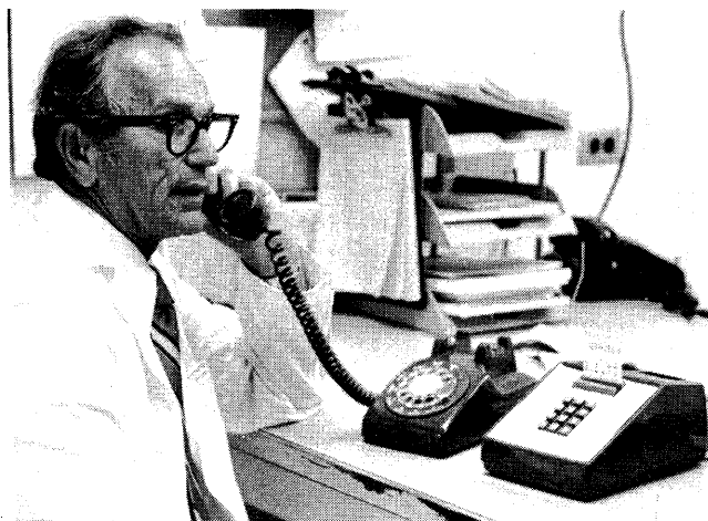
Figure 2—Photograph demonstrating the Touch-One, Card-Dialer pad attached to a conventional rotary telephone. Note the insertion of the patients' Dial-A-Card in the reader. The physician is either ordering tests or listening to laboratory results.
