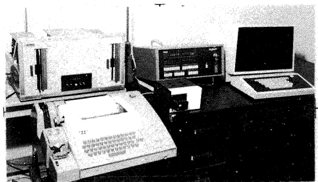
Figure 3—A disk-based microcomputer development system
