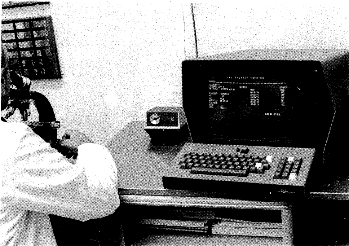
Figure 4—Note the availability of a CRT at the pathologist's microscope work-bench allowing him to retrieve the total PMF and Quality Control data thus allowing correlation between the anatomic findings with clinical pathology data.
