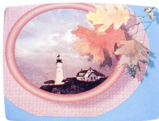
Using scissors mode, the leaves are grabbed from the camera stand and inserted over lighthouse; the low opacity shadow behind the leaves was added using a luminance key.
