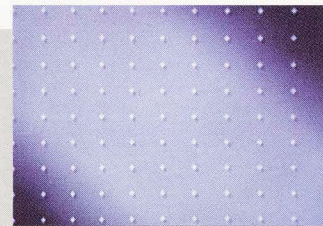
Used as a key signal, the grid is luminance keyed with a drop shadow onto a gradated background.
