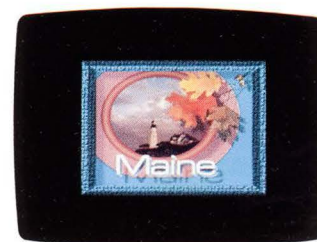
Using an effect while in playlist, the entire framed graphic is reduced in size with a key signal of the same proportion. Dissolves and wipes can take place within the reduced area.
