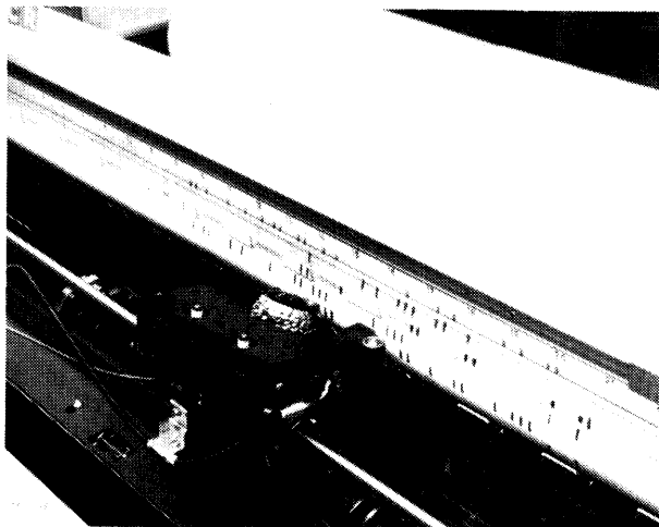
The NCR 299's simplicity and adaptability are demonstrated by the ease with which it can be programmed. A narrative Program Coding Form is filled in by the operator, and then is transferred to the bar-coded Program Assembly Card by means of a pencil. The marks on the Program Assembly Card are read by the optical scanner, which is shown in its reading position. The penciled marks are read by the scanner and converted to electrical impulses, which are then sent to the computer's memory and stored as a usable program.
