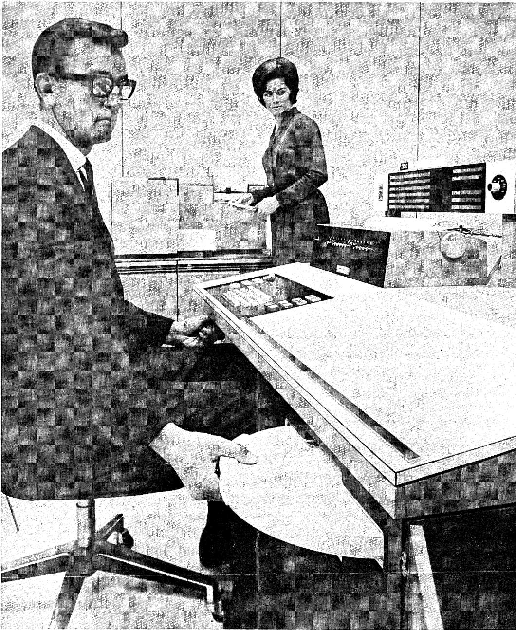
IBM 1130 Computing System, showing the disc cartridge (lower right) and the 1442 Card Read Punch (at rear).
