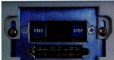
Maintenance panel provides access to powerful diagnostics.
