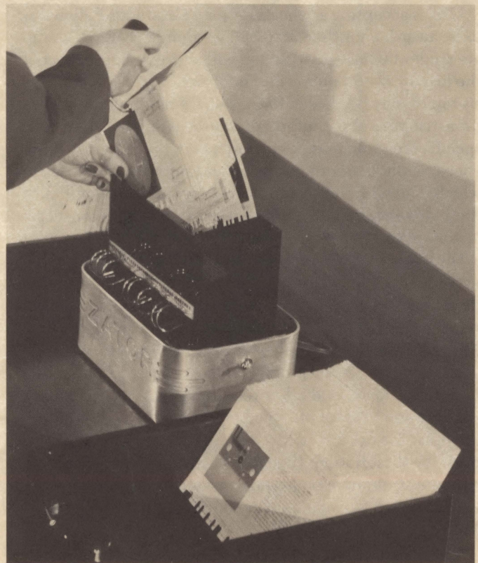
A demonstration of Zatocoding, a punched card information retrieval system developed by Calvin N. Mooers in 1947. The photograph is part of a large collection of records recently donated to CBI by Mooers with the assistance of the Massachusetts Institute of Technology Archives. The collection includes the records of the Zator Company, as well as Mooers' personal records.
