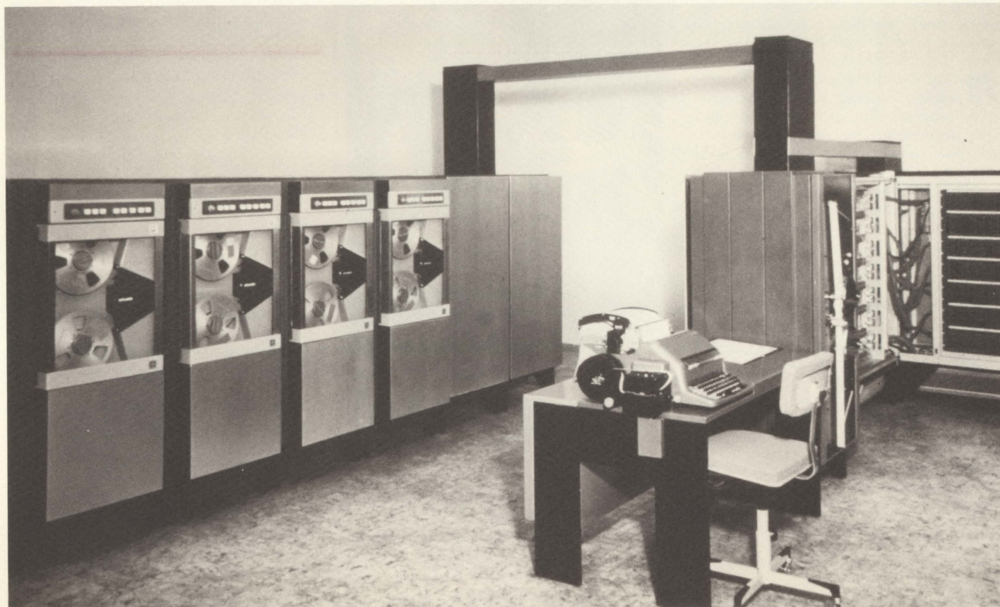
A photograph of the Olivetti Elea 6001 at the Università degli Studi di Pavia. The 6001 became available in 1961 and was sold as a transistorized, scientific computer. The photograph was donated to CBI from Olivetti.
