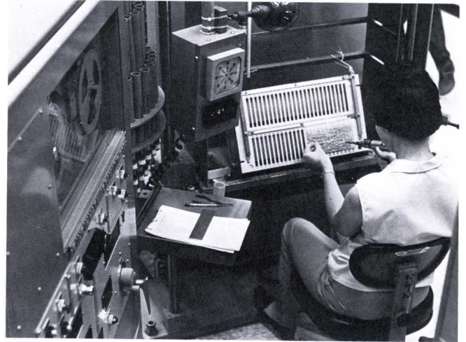
Cincinnati-designed NC wiring machine.
