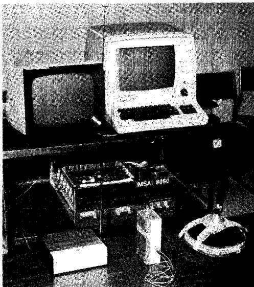
Fig. 2A. Components of the ultrasonic locator system for blind mobility tracking. The RF receiver is the small box in the center foreground with its trailing antenna. This receiver is generally worn on the belt of the blind pedestrian. The ultrasonic transmitter is shown in the right foreground as a small omnidirectional ultrasonic loudspeaker mounted on a lightweight headband worn by the pedestrian being tracked. The RF transmitter is in the left foreground and the IMSAI 8080 microcomputer in the lower background. The control terminal on the right and the output display graphics monitor is on the left. The blind pedestrian's path is traced out in detail on this monitor. The sequential coordinates of this path are stored in memory and subsequently dumped onto a cassette recorder (not shown) when the 64K memory is full.
