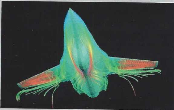
Streamlines over a modified F-16 configuration courtesy NASA Ames Research Center.
