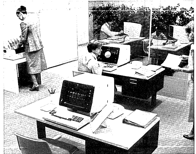
The 3270 permits up to 32 users to simultaneously access host facilities. While designed primarily for inquiry/update applications, users may attach personal computers to off-load processing from the mainframe.
