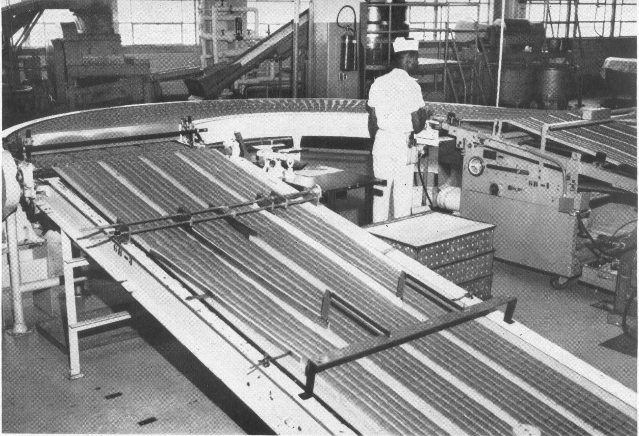
Stacked end to end, these Fig Newton cakes would reach from New York to Philadelphia. More than one million pounds are baked daily, using a process computer to direct batching of the ingredients.
