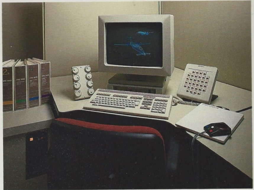
The PS 390 displays dynamic, anti-aliased wireframe images and locally computed shaded images on a single raster display. This model was created using GEOMOD™, part of the I-DEAS™ package from SDRC.
