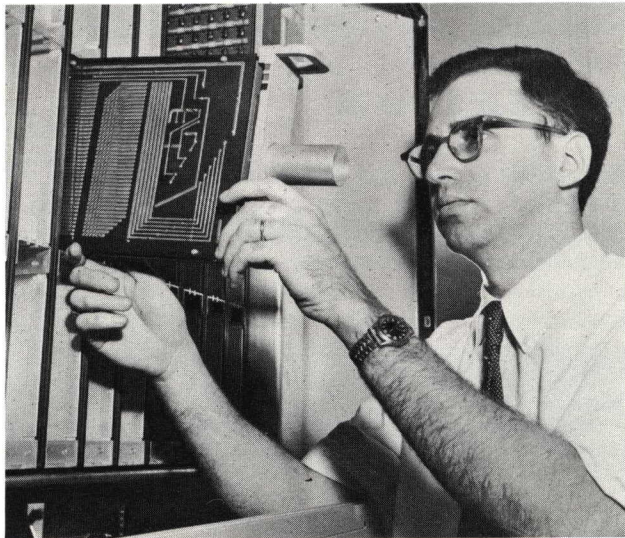
Unit package techniques, used throughout the system, insure high reliability and facilitate maintenance.
