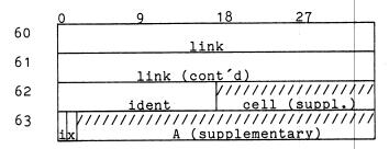
There is still some wasted storage here ('ident', 'i', and 'x' could all fit in one word), but elimination of that waste would require a change in the level structure of the variable.
