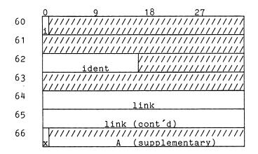
This wasteful layout arises from the fact that 'link' is an aligned 'pointer' and specifies an even word boundary not only for its own storage, but also for the structure 'A.cell' of which it is a member and for the structure 'A' which, in turn, contains 'A.cell'.
