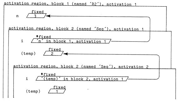
The storage unit for the parameter, 'i', is given the data type '\*fixed' to show that it holds a pointer to a 'fixed' storage unit. Because 'i' is a parameter, a reference to 'i' is interpreted as a reference to the storage unit designated by the pointer. The arrows in the diagram show how each parameter designates and argument storage unit. The storage unit designated '(temp)' is a system temporary used for the value of 'i-1' in the second 'call' statement in the program.
