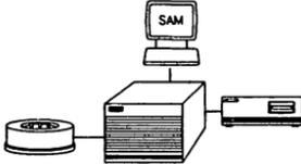
The diagram illustrates the fbackup setup. A monitor labeled 'SAM' is connected to a central server unit. The server unit is connected to a tape drive, which is connected to a DAT/DDS tape.
