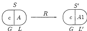
Figure 5: The CHARM rewrite rule for the agent A = \text{ask}(c) \rightarrow A1 .
