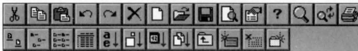
Figure 5-3. Images in the two standard bitmaps provided by the common control DLL.
