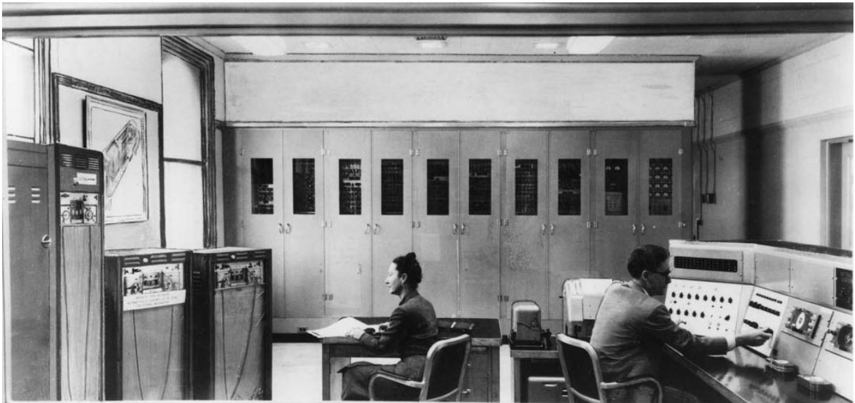
Fig. 1. SEAC, showing the magnetic tapes and wire cartridges, the operators console, and the racks of logic circuitry.
