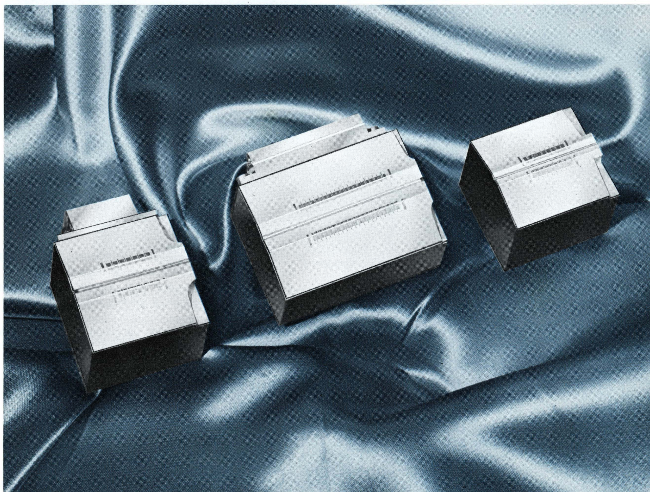
Figure 1—POTTER Standard Read/Write Head Assemblies. (Photo shows 7, 21 and 9-track heads, l. to r.)
