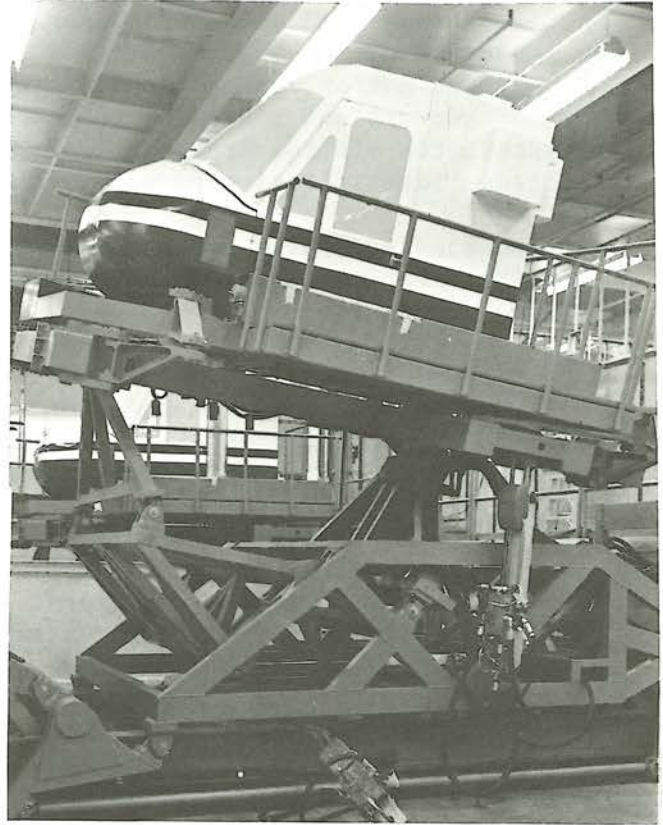
one of the four-cockpit SFTS Complex during in-plant test
