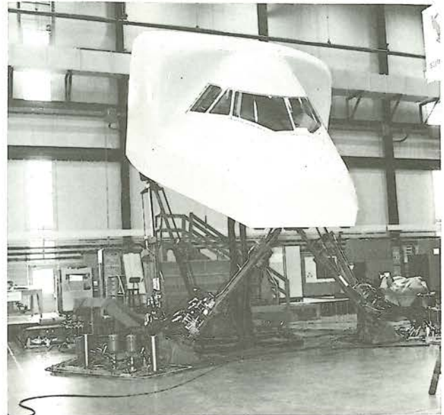
Simulator on Six-Degree Motion System
