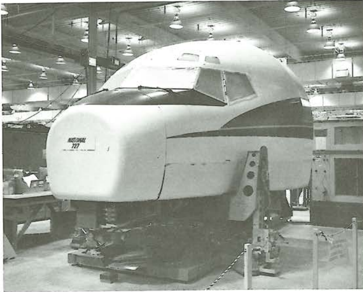
727 Simulator on Three-Degree-of-Freedom System
