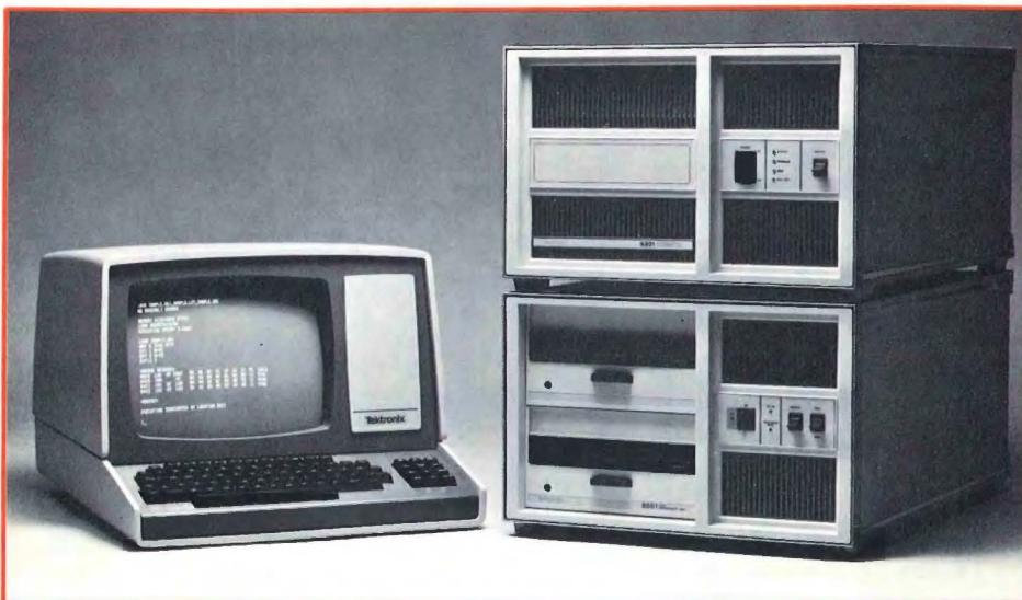
Fig. 1. The 8550 Microcomputer Development Lab is a versatile software development and hardware/software integration system for microprocessor-based product design. The system supports many popular 8- and 16-bit microprocessors.
