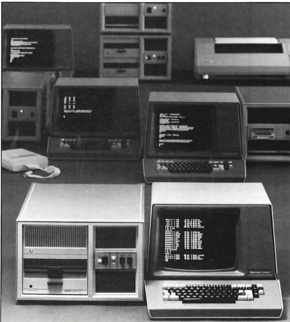
Figure 1. The Tektronix 8560 Multi-User Software Development Unit (lower left) accommodates up to eight workstations, including multiple 8540 Integration Units and line printers.
