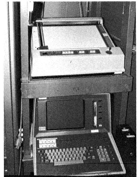
Inside the screen room, the data is fed to the Tektronix 4051 and printed on the 4662.
