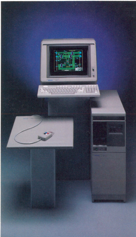
A TekniCAD configuration could include a Tektronix color raster 4107 or a 4109 Computer Display Terminal paired with the Tektronix 4170 Local Graphics Processing Unit and an optional 4957 Graphics Tablet.
