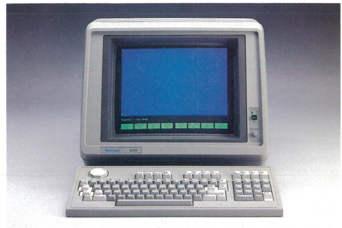
Figure 4. The key labels on the 4105 display identify the top layer of the interface hierarchy: the major tools within the system. Pressing the corresponding key on the 4105 keyboard will select that tool.
