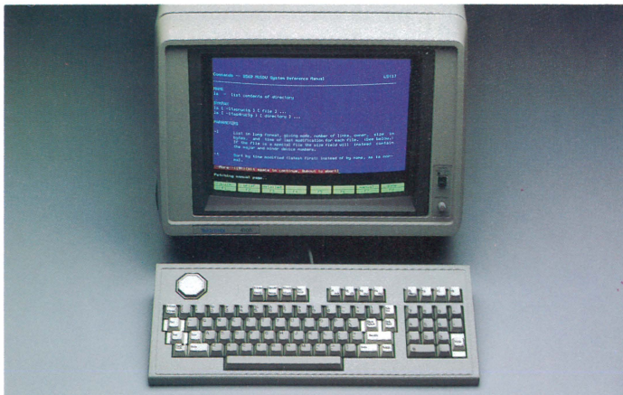
Figure 1. Functional areas of the 4105 display are readily discernible by their colors.
