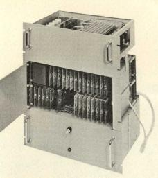
These ingenious self-contained, transistorized memories, introduced by Telemeter Magnetics, provide means for synchronizing data systems of different speeds. Their operation is analogous to a computer having a simple, predetermined program. There are three basic types of buffers-sequential buffers, conversion buffers, and random access buffers.
