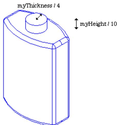
To position the cylinder, you need to define a coordinate system with the *gp\_Ax2* class defining a right-handed coordinate system from a point and two directions - the main (Z) axis direction and the X direction (the Y direction is computed from these two). To align the neck with the center of the top face, being in the global coordinate system (0, 0, *myHeight*), with its normal on the global Z axis, your local coordinate system can be defined as follows:
