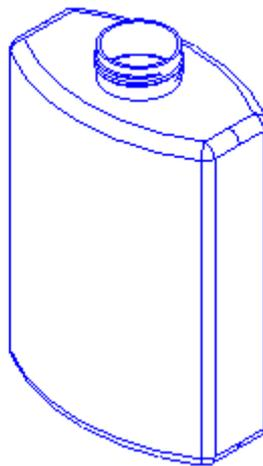
In the tutorial we will create, step-by-step, a function that will model a bottle as shown above. You will find the complete source code of this tutorial, including the very function *MakeBottle* in the distribution of Open CASCADE Technology. The function body is provided in the file `samples/qt/Tutorial/src/MakeBottle.cxx`.
