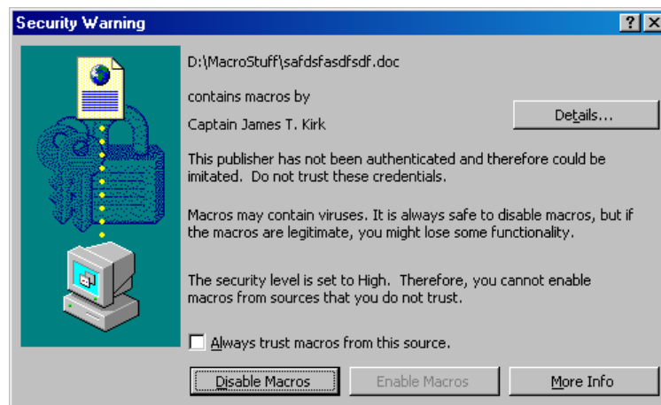
Figure 3-2: Security Warning dialog box in Office 2000. This is what the user sees when security is set to high or medium and the user attempts to open a signed document from a source that has not yet been trusted on that computer.
