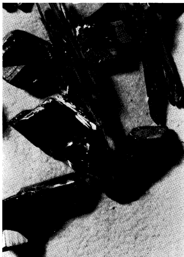
Figure 3 Needles and more equidimensional crystals of (\text{SN})_x .
